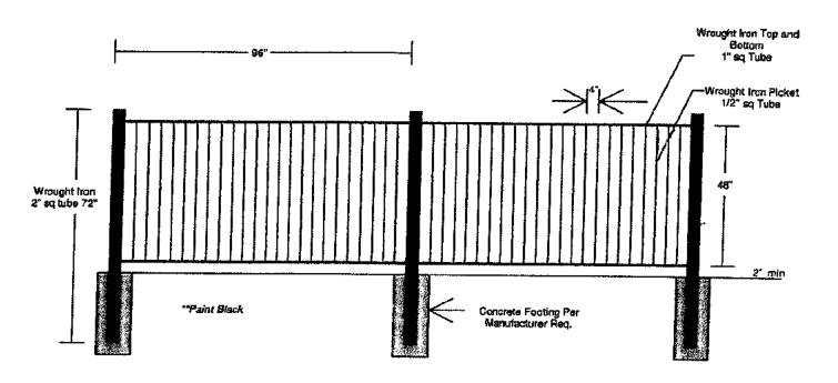
POWDER COATED TUBULAR STEEL WHICH SHALL HAVE A BLACK FINISH, RUST RESISTANT PAINT, FORTH-EIGHT INCHES (48") IN HEIGHT MAY BE USED IN LIEU OF WROUGHT IRON. THE FULL WIDTH OF THE REAR LOT LINE SHALL BE WROUGHT IRON OR TUBULAR STEEL. REFER TO SECTION 1.2.4 OF THE DESIGN GUIDELINES FOR MORE INFORMATION.
