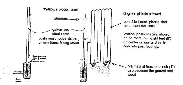
TOP RAIL REQUIRED. TRIM FOR SIDE AND REAR YARD FENCES NOT VISIBLE FROM THE STREET ARE OPTIONAL. ALL PORTIONS OF THE FENCE THAT MAY BE VIEWED FROM ANY STREET SHALL BE STAINED WITH THE COLOR SPECIFIED BELOW.
